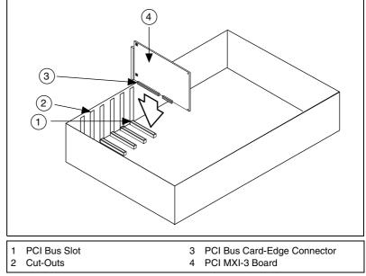
Figure 2-1. Installing the PCI MXI-3
